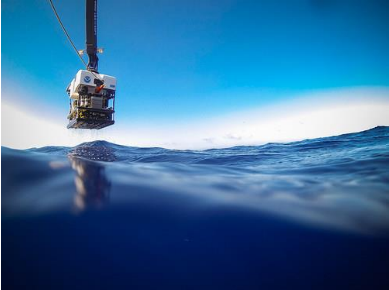
Remotely operated vehicle Deep Discoverer is recovered from a dive during an expedition. Credit: NOAA Okeanos Explorer Program, Gulf of Mexico 2014 Expedition.
